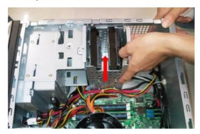
**4.4** Disconnect the eight screws fixed in HDD cage side.
